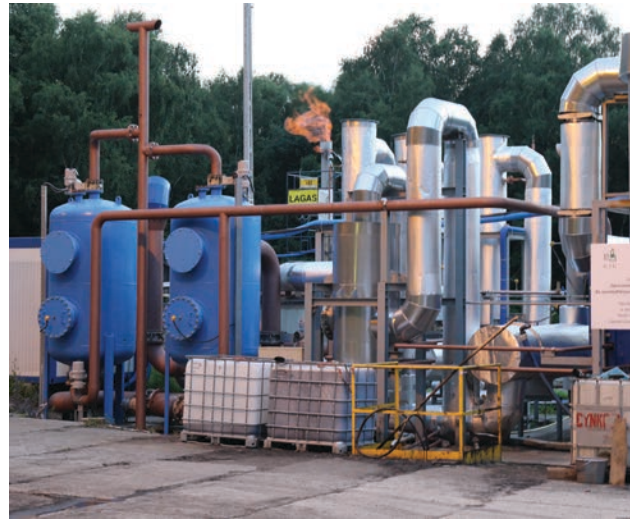
Fig. Installation for pressure simulation of the underground coal gasification process
